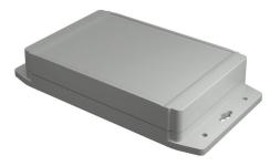
Hammond enclosure, NEMA 4/4X/6/6P/12/13, 180 x 121 x 38mm (HxWxD), integral mounting flange, polycarbonate, RAL 7035 light gray, screw cover, purchase subpanel separately.
