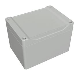
Hammond enclosure, NEMA 4/4X/6/6P/12/13, 120 x 90 x 81mm (HxWxD), ABS plastic, RAL 7035 light gray, screw cover with smooth recess, purchase subpanel separately.
