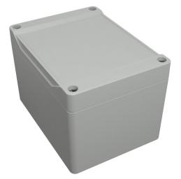
Hammond enclosure, NEMA 4/4X/6/6P/12/13, 120 x 90 x 81mm (HxWxD), polycarbonate, RAL 7035 light gray, screw cover with smooth recess, purchase subpanel separately.
