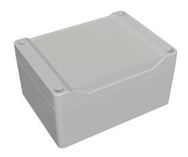
Hammond enclosure, NEMA 4/4X/6/6P/12/13, 120 x 90 x 61mm (HxWxD), ABS plastic, RAL 7035 light gray, screw cover with smooth recess, purchase subpanel separately.
