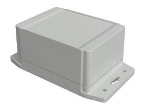
Hammond enclosure, NEMA 4/4X/6/6P/12/13, 120 x 91 x 63mm (HxWxD), integral mounting flange, ABS plastic, RAL 7035 light gray, screw cover, purchase subpanel separately.
