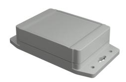
Hammond enclosure, NEMA 4/4X/6/6P/12/13, 120 x 91 x 38mm (HxWxD), integral mounting flange, polycarbonate, RAL 7035 light gray, screw cover, purchase subpanel separately.
