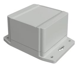
Hammond enclosure, NEMA 4/4X/6/6P/12/13, 90 x 90 x 63mm (HxWxD), integral mounting flange, ABS plastic, RAL 7035 light gray, screw cover, purchase subpanel separately.
