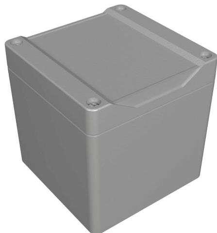
Hammond enclosure, NEMA 4/4X/6/6P/12/13, 90 x 90 x 91mm (HxWxD), polycarbonate, RAL 7035 light gray, screw cover with smooth recess, purchase subpanel separately.
