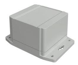
Hammond enclosure, NEMA 4/4X/6/6P/12/13, 90 x 90 x 63mm (HxWxD), integral mounting flange, polycarbonate, RAL 7035 light gray, screw cover, purchase subpanel separately.
