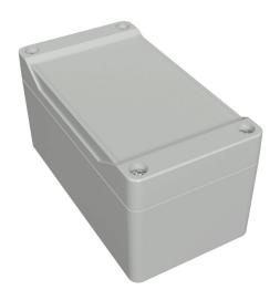
Hammond enclosure, NEMA 4/4X/6/6P/12/13, 120 x 65 x 61mm (HxWxD), ABS plastic, RAL 7035 light gray, screw cover with smooth recess, purchase subpanel separately.
