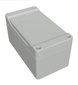
Hammond enclosure, NEMA 4/4X/6/6P/12/13, 120 x 65 x 61mm (HxWxD), ABS plastic, RAL 7035 light gray, screw cover with smooth recess, purchase subpanel separately.
