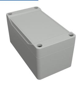
Hammond enclosure, NEMA 4/4X/6/6P/12/13, 120 x 65 x 61mm (HxWxD), polycarbonate, RAL 7035 light gray, screw cover with smooth recess, purchase subpanel separately.
