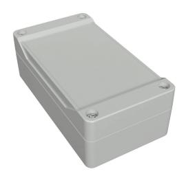
Hammond enclosure, NEMA 4/4X/6/6P/12/13, 120 x 65 x 41mm (HxWxD), ABS plastic, RAL 7035 light gray, screw cover with smooth recess, purchase subpanel separately.
