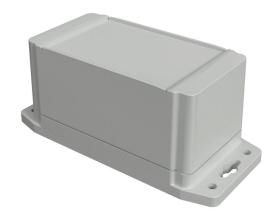
Hammond enclosure, NEMA 4/4X/6/6P/12/13, 120 x 66 x 63mm (HxWxD), integral mounting flange, ABS plastic, RAL 7035 light gray, screw cover, purchase subpanel separately.
