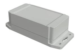
Hammond enclosure, NEMA 4/4X/6/6P/12/13, 120 x 66 x 43mm (HxWxD), integral mounting flange, ABS plastic, RAL 7035 light gray, screw cover, purchase subpanel separately.
