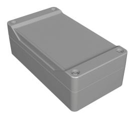
Hammond enclosure, NEMA 4/4X/6/6P/12/13, 120 x 65 x 41mm (HxWxD), polycarbonate, RAL 7035 light gray, screw cover with smooth recess, purchase subpanel separately.
