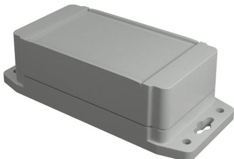
Hammond enclosure, NEMA 4/4X/6/6P/12/13, 120 x 66 x 43mm (HxWxD), integral mounting flange, polycarbonate, RAL 7035 light gray, screw cover, purchase subpanel separately.
