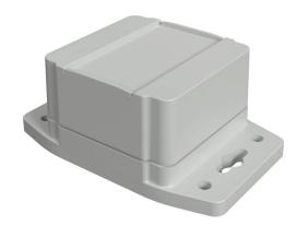
Hammond enclosure, NEMA 4/4X/6/6P/12/13, 65 x 65 x 43mm (HxWxD), integral mounting flange, ABS plastic, RAL 7035 light gray, screw cover, purchase subpanel separately.
