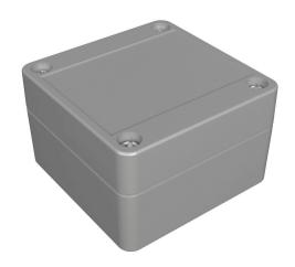
Hammond enclosure, NEMA 4/4X/6/6P/12/13, 65 x 65 x 41mm (HxWxD), polycarbonate, RAL 7035 light gray, screw cover with smooth recess, purchase subpanel separately.
