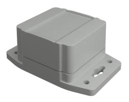
Hammond enclosure, NEMA 4/4X/6/6P/12/13, 65 x 65 x 43mm (HxWxD), integral mounting flange, polycarbonate, RAL 7035 light gray, screw cover, purchase subpanel separately.
