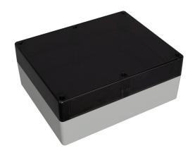
Hammond enclosure, NEMA 4/4X/6/6P/12/13, 299 x 240 x 120mm (HxWxD), polycarbonate, RAL 7035 light gray, smoke polycarbonate screw cover, purchase subpanel separately.
