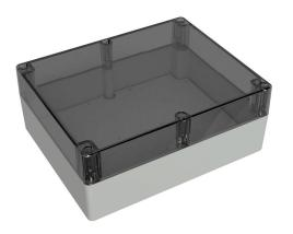
Hammond enclosure, NEMA 4/4X/6/6P/12/13, 299 x 240 x 120mm (HxWxD), polycarbonate, RAL 7035 light gray, clear polycarbonate screw cover, purchase subpanel separately.
