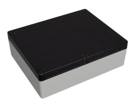
Hammond enclosure, NEMA 4/4X/6/6P/12/13, 299 x 240 x 95mm (HxWxD), polycarbonate, RAL 7035 light gray, smoke polycarbonate screw cover, purchase subpanel separately.
