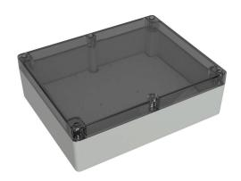
Hammond enclosure, NEMA 4/4X/6/6P/12/13, 299 x 240 x 95mm (HxWxD), polycarbonate, RAL 7035 light gray, clear polycarbonate screw cover, purchase subpanel separately.
