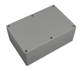
Hammond enclosure, NEMA 4/4X/6/6P/12/13, 299 x 200 x 120mm (HxWxD), polycarbonate, RAL 7035 light gray, screw cover, purchase subpanel separately.
