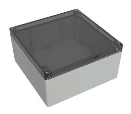
Hammond enclosure, NEMA 4/4X/6/6P/12/13, 180 x 180 x 90mm (HxWxD), polycarbonate, RAL 7035 light gray, clear polycarbonate screw cover, purchase subpanel separately.
