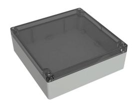
Hammond enclosure, NEMA 4/4X/6/6P/12/13, 180 x 180 x 60mm (HxWxD), polycarbonate, RAL 7035 light gray, clear polycarbonate screw cover, purchase subpanel separately.
