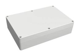
Hammond enclosure, NEMA 4/4X/6/6P/12/13, 240 x 160 x 60mm (HxWxD), polycarbonate, RAL 7035 light gray, screw cover, purchase subpanel separately.
