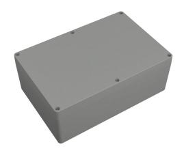
Hammond enclosure, NEMA 4/4X/6/6P/12/13, 240 x 160 x 90mm (HxWxD), polycarbonate, RAL 7035 light gray, screw cover, purchase subpanel separately.
