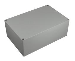
Hammond enclosure, NEMA 4/4X, 240 x 160 x 91mm (HxWxD), polycarbonate, RAL 7035 light gray, screw cover, purchase subpanel separately.
