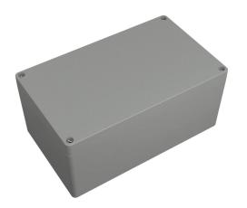
Hammond enclosure, NEMA 4/4X/6/6P/12/13, 200 x 120 x 91mm (HxWxD), polycarbonate, RAL 7035 light gray, screw cover, purchase subpanel separately.
