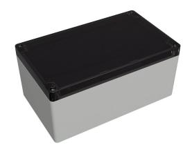
Hammond enclosure, NEMA 4/4X/6/6P/12/13, 200 x 120 x 91mm (HxWxD), polycarbonate, RAL 7035 light gray, smoke polycarbonate screw cover, purchase subpanel separately.
