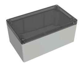
Hammond enclosure, NEMA 4/4X/6/6P/12/13, 200 x 120 x 91mm (HxWxD), polycarbonate, RAL 7035 light gray, clear polycarbonate screw cover, purchase subpanel separately.
