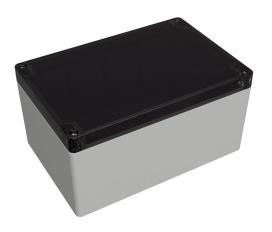
Hammond enclosure, NEMA 4/4X/6/6P/12/13, 180 x 120 x 91mm (HxWxD), polycarbonate, RAL 7035 light gray, smoke polycarbonate screw cover, purchase subpanel separately.
