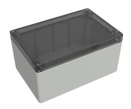
Hammond enclosure, NEMA 4/4X/6/6P/12/13, 180 x 120 x 91mm (HxWxD), polycarbonate, RAL 7035 light gray, clear polycarbonate screw cover, purchase subpanel separately.
