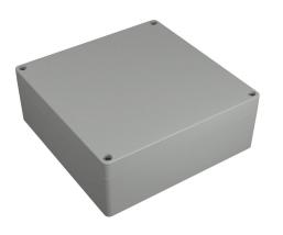
Hammond enclosure, NEMA 4/4X/6/6P/12/13, 160 x 160 x 61mm (HxWxD), polycarbonate, RAL 7035 light gray, screw cover, purchase subpanel separately.
