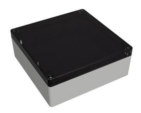
Hammond enclosure, NEMA 4/4X/6/6P/12/13, 160 x 160 x 61mm (HxWxD), polycarbonate, RAL 7035 light gray, smoke polycarbonate screw cover, purchase subpanel separately.
