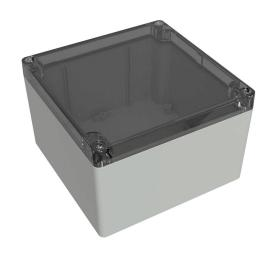
Hammond enclosure, NEMA 4/4X/6/6P/12/13, 140 x 140 x 90mm (HxWxD), polycarbonate, RAL 7035 light gray, clear polycarbonate screw cover, purchase subpanel separately.
