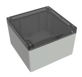
Hammond enclosure, NEMA 4/4X/6/6P/12/13,  $140 \times 140 \times 90$ mm (HxWxD), polycarbonate, RAL 7035 light gray, clear polycarbonate screw cover, purchase subpanel separately.
