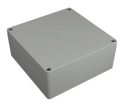
Hammond enclosure, NEMA 4/4X/6/6P/12/13, 140 x 140 x 60mm (HxWxD), polycarbonate, RAL 7035 light gray, screw cover, purchase subpanel separately.
