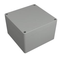
Hammond enclosure, NEMA 4/4X/6/6P/12/13, 120 x 120 x 80mm (HxWxD), polycarbonate, RAL 7035 light gray, screw cover, purchase subpanel separately.
