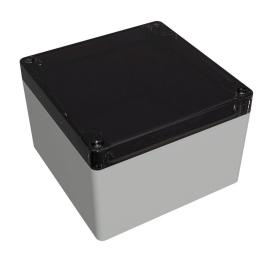
Hammond enclosure, NEMA 4/4X/6/6P/12/13, 120 x 120 x 80mm (HxWxD), polycarbonate, RAL 7035 light gray, smoke polycarbonate screw cover, purchase subpanel separately.
