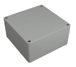
Hammond enclosure, NEMA 4/4X/6/6P/12/13, 120 x 120 x 61mm (HxWxD), polycarbonate, RAL 7035 light gray, screw cover, purchase subpanel separately.
