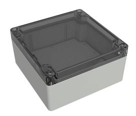
Hammond enclosure, NEMA 4/4X/6/6P/12/13,  $120 \times 120 \times 61$ mm (HxWxD), polycarbonate, RAL 7035 light gray, clear polycarbonate screw cover, purchase subpanel separately.
