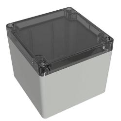
Hammond enclosure, NEMA 4/4X/6/6P/12/13, 105 x 105 x 90mm (HxWxD), polycarbonate, RAL 7035 light gray, clear polycarbonate screw cover, purchase subpanel separately.
