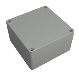
Hammond enclosure, NEMA 4/4X/6/6P/12/13, 105 x 105 x 60mm (HxWxD), polycarbonate, RAL 7035 light gray, screw cover, purchase subpanel separately.
