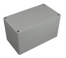
Hammond enclosure, NEMA 4/4X/6/6P/12/13, 160 x 90 x 91mm (HxWxD), polycarbonate, RAL 7035 light gray, screw cover, purchase subpanel separately.
