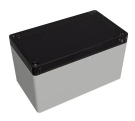
Hammond enclosure, NEMA 4/4X/6/6P/12/13, 160 x 90 x 91mm (HxWxD), polycarbonate, RAL 7035 light gray, smoke polycarbonate screw cover, purchase subpanel separately.
