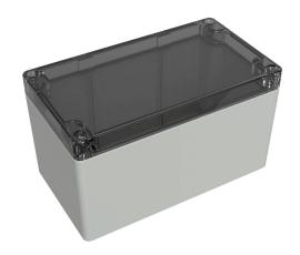
Hammond enclosure, NEMA 4/4X/6/6P/12/13, 160 x 90 x 91mm (HxWxD), polycarbonate, RAL 7035 light gray, clear polycarbonate screw cover, purchase subpanel separately.
