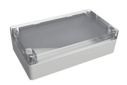
Hammond enclosure, NEMA 4/4X/6/6P/12/13,  $160 \times 90 \times 46mm$  (HxWxD), polycarbonate, RAL 7035 light gray, clear polycarbonate screw cover, purchase subpanel separately.
