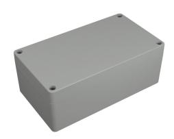
Hammond enclosure, NEMA 4/4X/6/6P/12/13, 160 x 90 x 61mm (HxWxD), polycarbonate, RAL 7035 light gray, screw cover, purchase subpanel separately.
