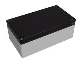
Hammond enclosure, NEMA 4/4X/6/6P/12/13, 160 x 90 x 61mm (HxWxD), polycarbonate, RAL 7035 light gray, smoke polycarbonate screw cover, purchase subpanel separately.
